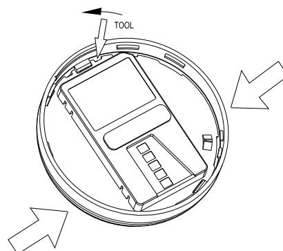
Remove the cover, open the sensor chamber and carefully clean it.
