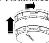
The detectors have a locking system to help prevent unauthorised detector removal. As supplied, the detectors can be removed without use of an extraction tool (useful for high ceilings).
