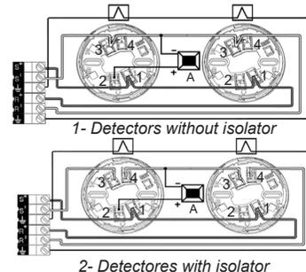
In case of installation of a warning action light is also necessary to respect the polarity of the installation as shown on the previous scheme.
