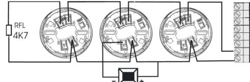
In case of installation of a warning action light is necessary to respect the polarity of the installation as shown on the previous scheme. The fire alarm control panel used on the installation must be current limited to 100 mA.
