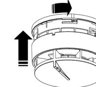
The detectors have a locking system to help prevent unauthorised detector removal. As supplied, the detectors can be removed without use of an extraction tool (useful for high ceilings).
